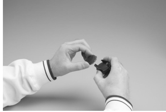
Figure 14: Removal of Filter from Filter Cover
