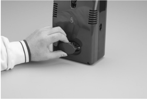
Figure 13: Removal of Air Intake Filter Cover
