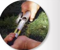
Simply turn the screw to release the coupling sleeve and then exchange the attachment.
