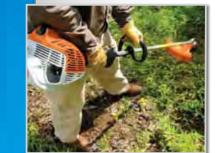
Straight shaft trimmers are the choice of lawn care professionals and large property owners. They are known to manage heavier brush and thicker weeds better than curved shaft models. Straight shaft trimmers have more reach and some can interchange cutting attachments like metal blades to offer enhanced versatility. Taller individuals enjoy the extended length of the shaft. For the avid user bike handles are also available.
