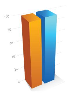
**R61691T (10 micron): 99%,** *SAE J1839 OCT2010, Coarse Droplet Water / Fuel Separation Test @ 150 GPH with ULSD*
