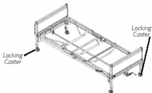
Figure 4B: Locking Caster positioning
