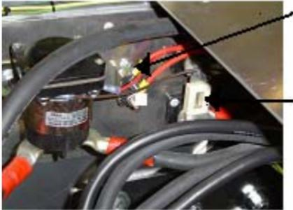
Front Controls Fuse - This fuse is for the front controls of the vehicle (key switch, converter, heater, etc). It is a 30 amp fuse (NON-30).
