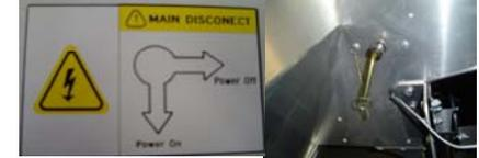
This switch should be disengaged before any maintenance is performed on the vehicle.
