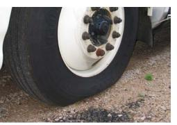
pressures were checked while the vehicle was parked at the yard, running over a nail 20 feet outside the gate can lead to a low tire pressure. This is why automatic tire inflation systems are so popular on trailers. Air is automatically added as the vehicle is running down the highway whenever the pressure drops below the system's control box setting.
