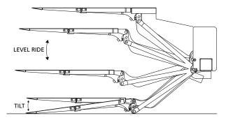
when in the raising and lowering mode. The platform tilts when it makes contact with the ground to provide
