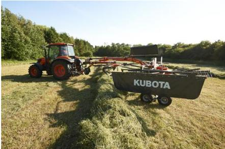
All functions can be controlled from the tractor cab. A simple pull of a rope is all that is needed to activate the standard hydraulic lifting of the swath board. And with a 20" lifting height, swaths are easily crossed.
