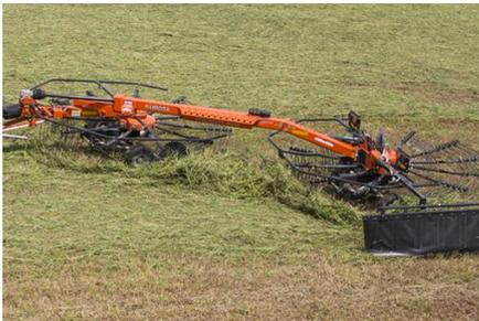
Up to twelve tangential tine arms and four double tines per arm provide high tine frequency to ensure clean raking performance – even at reduced rpm and high travel speed. Infinitely variable cam track adjustment allows fine-tuning to obtain optimum raking and swath formation according to crop conditions.
