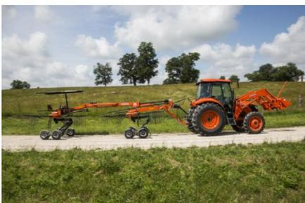
There's no need to remove tine arms when converting the RA2071T into transport position. The swath board is lifted hydraulically and transport width is reduced to 9'10" (to reach 8'1" the tine arms can be removed).
