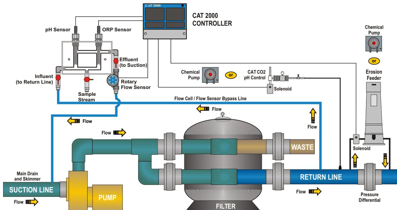
**ALL CHEMICALS MUST BE INJECTED DOWN STREAM FROM HEATER & FLOW CELL**
