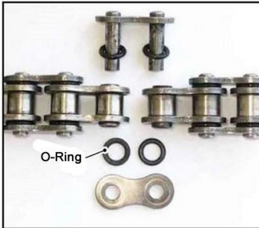
Chains are characterized by two key parameters: Pitch Length and Link Internal Width. There's an international standard that uses a 3-digit code to indicate these two values (for example: 415, 420, 428, 520, 525, 530) marked on the outer link plate.
