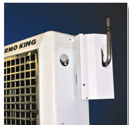
PDPF installs in place of the muffler on SB units, externally on Super II (shown)
