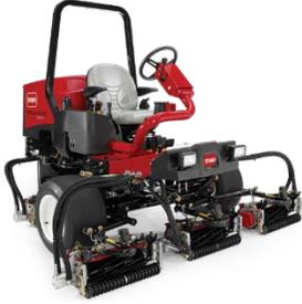
This model is very similar to our 3575-D/3555-D models as far as engine size and our 3-wheel traction unit with slick tires, but comes in an 82" width of cut only using 5" diameter cutting units. This unit will cut both warm and cool season turf on fairways, approaches or large multiple tee boxes.
