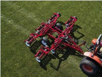
Last but not least, is our ground drive Reelmaster 11, 7 or 5 Blade Cutting Units, which can also be used in mowing of fairways or roughs. **The 5 unit frame has a mowing width of 11' or the 7 unit frame with a mowing width of 14.4'**. These 2 units can cover a lot of ground, giving the customer an economical option when it comes to mowing.
