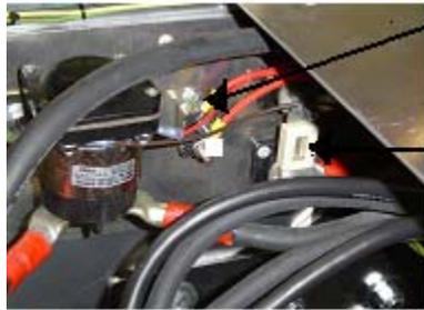
1. The main fuse for the 72 volt system which has 325 amps is located in the back of the machine on the left side wall.
