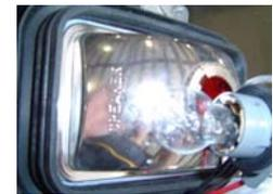
3. Twist the bulb to disconnect.
