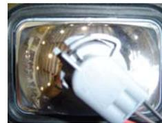
2. Turn the connector counter-clockwise to unhook.
