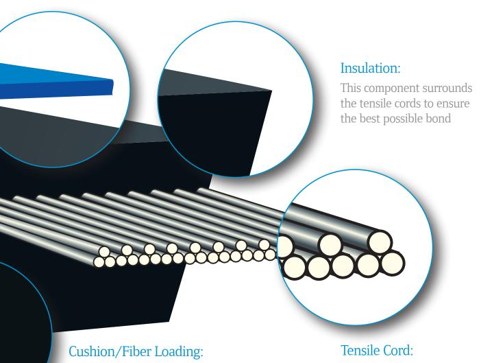
Provides the necessary support for the cords, preventing distortion and collapsing of the belt. It provides unidirectional support which helps resists abrasion, reduces noise and controls the coefficient of friction.
