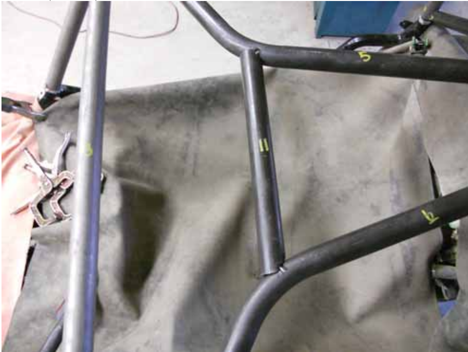
20. INSTALL 11 BAR (MID SPREADER) BETWEEN 5 AND 6 AND TACK WELD.
