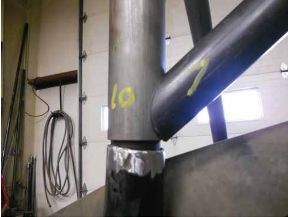
20. INSTALL 11 BAR (MID SPREADER) BETWEEN 5 AND 6 AND TACK WELD.
